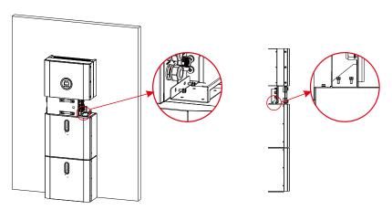
Figure 15 Inverter Installation on the Wall
