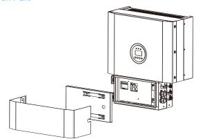
Figure 5 Inverter without Cable Box Covers- Front View
