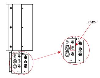
Figure 25 PV Wiring
