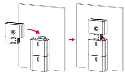
Figure 14 Inverter Installation
