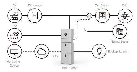
Figure 3 Hybrid-coupled Storage System - Scheme
