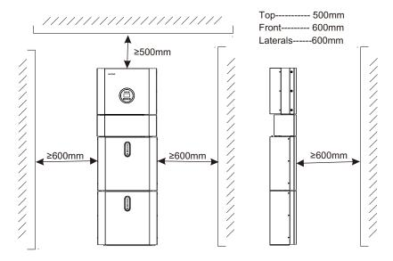
Figure 8 Limit Distance of Installation to Neighboring Objects
