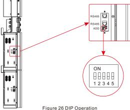
Step14 Open the front cover of the last battery and remove the DIP cover. Now set the DIP switch 2 to "on" mode and close the cover again.
