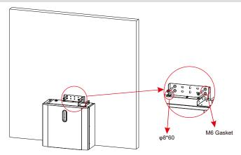
Figure 12 Battery Installation – Mounting on the Wall
