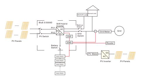
Figure 31 Hybrid-coupled system
