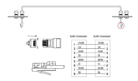
Figure 21 Network Cable Type B
