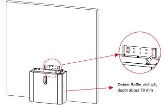
Figure 11 Battery Installation - Drill Holes
