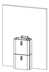
Figure 13 Battery Installation – Second Battery Installation
