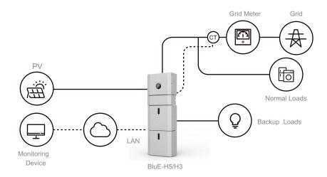
Figure1 DC-coupled Storage System – Scheme
