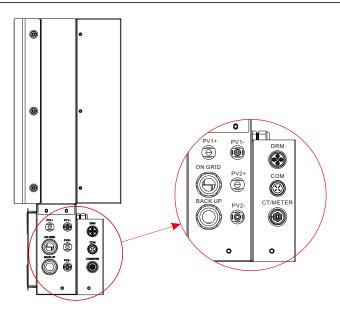
Figure 19 Cable Box Bottom View, Wiring Connectors
