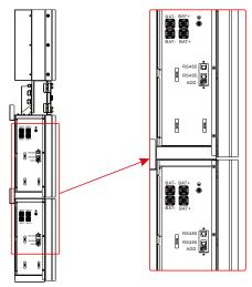
Figure 22 Wiring the Communication Cable
